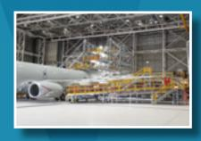
The P8 Maintenance Docking System has been specifically designed and built by Varley to facilitate scheduled deeper maintenance activities on the P-8A Poseidon aircraft and comprises fixed and mobile access and work platforms providing 240V Ac and 32V DC power and lighting, compressed and breathing air, air conditioning and fuel tank ventilation ducting, and integrated fall arrest and fall prevention.
